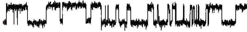
Figure 3.8 An RTS observed on a p-MOSFET, V_{GS} = -1.1 V, V_{DS} = 0.2 V (Arbitrary units along the X and Y axis). Note the distinction in the RTS level and the device background noise.
